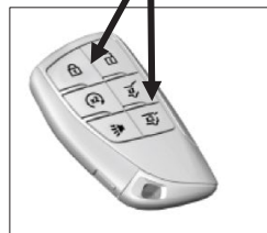
2 nd Row Passive entry button WILL unlock 2 nd Row door if Remote is present. A double press of either the remote fob Unlock button, or interior courtesy switch Lock/Unlock buttons will unlock all doors, including the liftgate.
