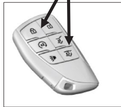
2 nd Row Passive entry button WILL unlock 2 nd Row door if Remote is present. A double press of either the remote fob Unlock button, or interior courtesy switch Lock/Unlock buttons will unlock all doors, including the liftgate.
