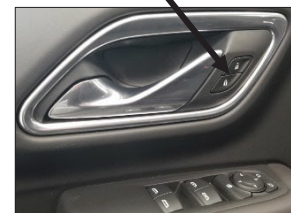
2 nd Row Passive entry button WILL unlock 2 nd Row door if Remote is present. A double press of either the remote fob Unlock button, or interior courtesy switch Lock/Unlock buttons will unlock all doors, including the liftgate.
