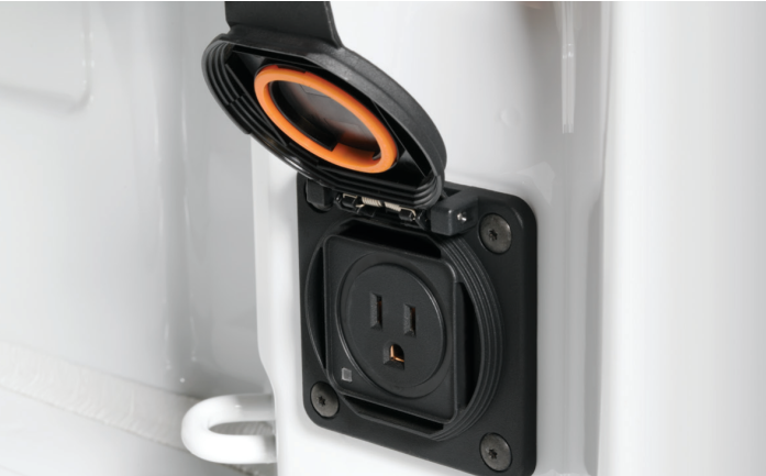
Standard 120-volt, 400 watt, 3.33 amp, power outlet in bed
