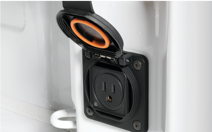
Standard 120-volt, 400 watt, 3.33 amp, power outlet in bed
