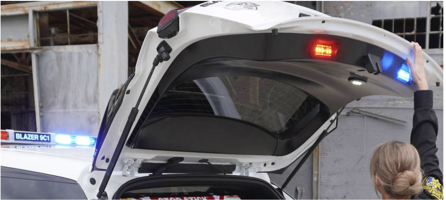
T53 REAR LIFTGATE WARNING LIGHTS
