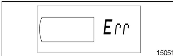
If more than one tire location contains the same sensor number, the display will prompt an error with the conflicting tires filled in and the associated sensor number. Press any button to return the tire selection menu and make necessary corrections.
