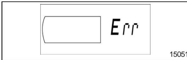
If more than one tire location contains the same sensor ID, the display will prompt an error and flash between this message and the display, with the conflicting tires filled in. If so indicated repeat the programming procedure above.
