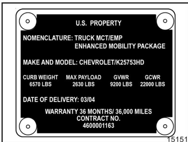
The data plate is used to inform the operator of the vehicle as to the make, model, Gross Vehicle Weight (GVW), payload and contract number after upfitting. It is located on the left inner door panel front.
