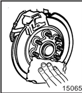
10. Remove any rust or dirt from the wheel bolts, mounting surfaces and spare wheel.
